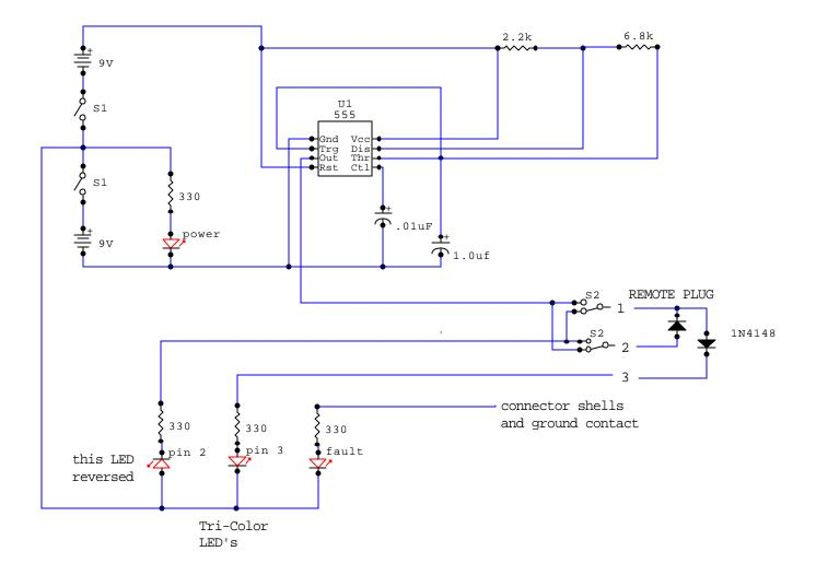
This is a slight modification of Farrel Becker's design. It has an LED added to show when the power is on. The numbers on the remote plug correspond to the pin designations of an XLR connector. The tester can also be used to test TRS TS and RCA connectors also.
